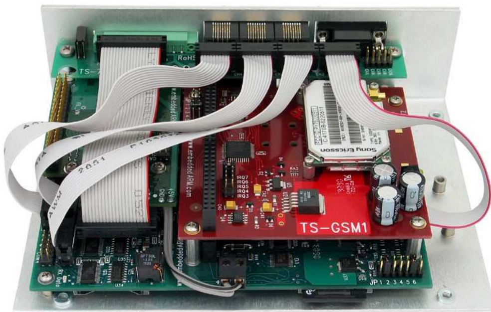
Internal view of TS-ENC730 shown with TS-7300, TS-732, TS-730C, TS-GSM1 and all the included cables
